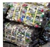
Collected PET bottles are crushed and packed into bales at the Seisō Center.
